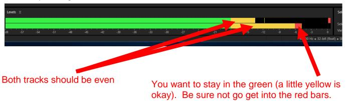
13. To adjust the gain turn the Channel 1 and 2 knobs on the M-AUDIO MoblePro box until you have a balanced, undistorted input. Record a short test track.
